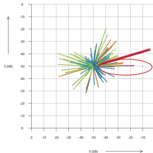
Fig. 12 Room 5 – near field monitors - desk reflection attenuated by absorption
