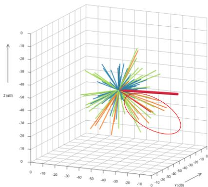
Fig. 10 Room 2 – near field monitors obscuring main monitors
