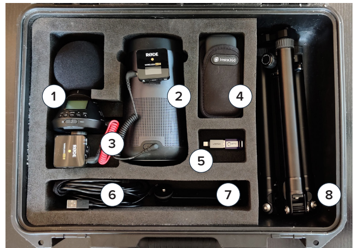
Recommended IRIS Mini kit: (1) Zoom H3-VR microphone, (2) Bose Revolve+ II speaker, (3) Rode Wireless Go wireless system, (4) optional 360° camera, (5) IRIS dongle, (6) charging cables, (7) tripod attachment, (8) MeFOTO RoadTrip Air tripod.
